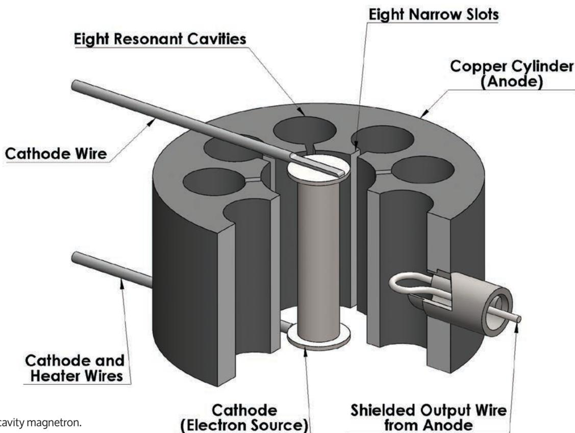
Cutaway of cavity magnetron.
